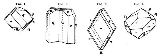
"The habit is shown in Fig. 1, but single crystals are rare, most crops consisting entirely of twinned crystals of the habit represented in Fig. 2. The twin plane is q(011). The mean angular values observed with seven of the twins were:
